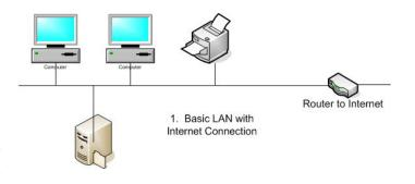
connects to the Internet. Internal to the LAN, data flows between the computers, printers, file server, and router using the ethernet protocol. Devices on the LAN are addressed in an IP address space called a netblock. The IP protocols are designed so that the router knows which devices are connected to the LAN and which are not. If the
